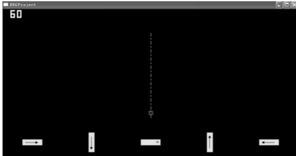
Fig. 2 The configuration of flicking targets: illustration of the BCI design used for performing geometric modeling (frequencies for flickering targets from left to right are 12, 10, 13, 15, and 14Hz)
